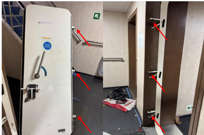
Figure 2: Visuals of the breached Citadel door and its hinges after the incident
