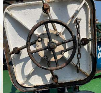
Damaged booby Hatch packing
