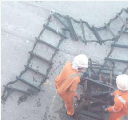
Starboard embarkation ladder, that had parted during lowering, being retrieved
