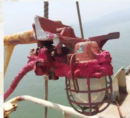
Embarkation light not working and damaged
