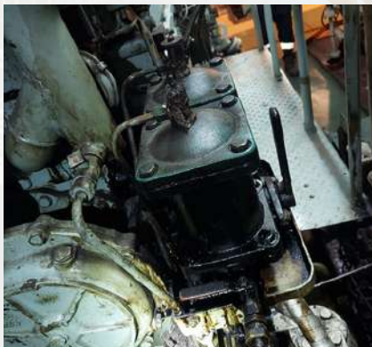
Leaking Fuel Oil from AE
