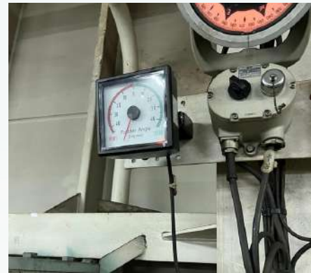
Defective Rudder angle indicator
