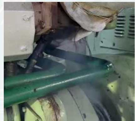
Exhaust leakage from A/E
