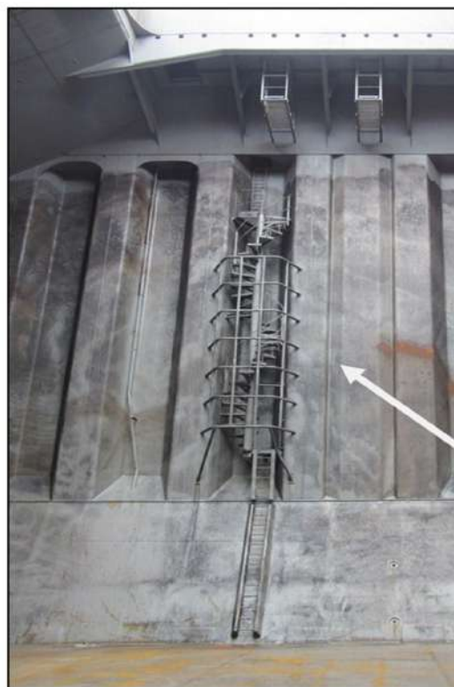
An Australian ladder on a bulk carrier, however, without the enclosing trunk. (Image for illustration purpose only)
