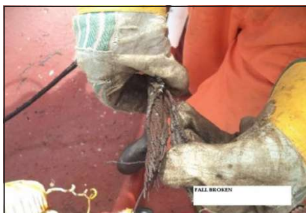
(Parted wire which was fitted as falls)
