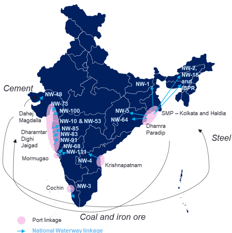
Figure 49: Strategic integration of National Waterways with coastal ports enables multimodal movement of coal, iron ore, cement, and steel across India
